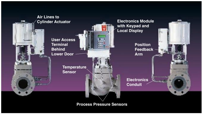
Figure 1: Valtek StarPac® II Intelligent Control System Components
