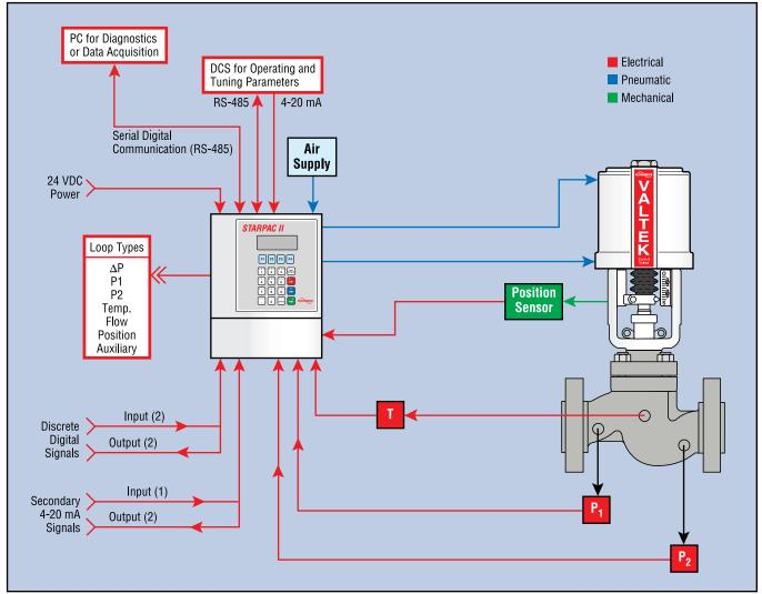
Figure 3: StarPac II Intelligent Control System Schematic
